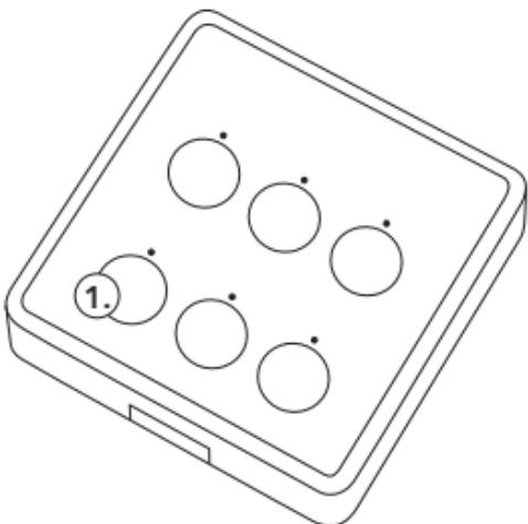
1. 6 individually configurable touch buttons with integrated LEDs
